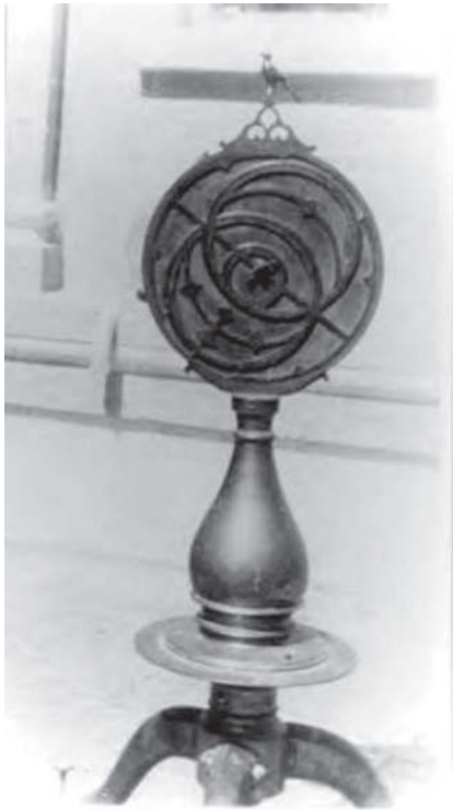
Fig. 7. Indo-Persian North-South Astrolabe, attributable to Bulhomal. Photo from the archives of the Museum of the History of Science, Oxford
