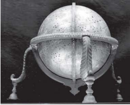
Fig. 13. Sanskrit Celestial Globe, attributable to Bulhomal. The zenith ring is mounted upside down. Butler Library, Columbia University, New York. Photo courtesy Butler Library
