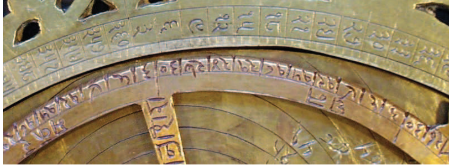
Figure 8: Above the Numerals on the Rim of the Mater; below the Numerals on the Rete
